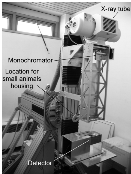
Fig. 1. The multi-energy X-ray system for small animals. The Bragg monochromator is located between the X-ray tube (on the top) and the detector (on the bottom). The gantry with rotational and translation axes is also shown.
