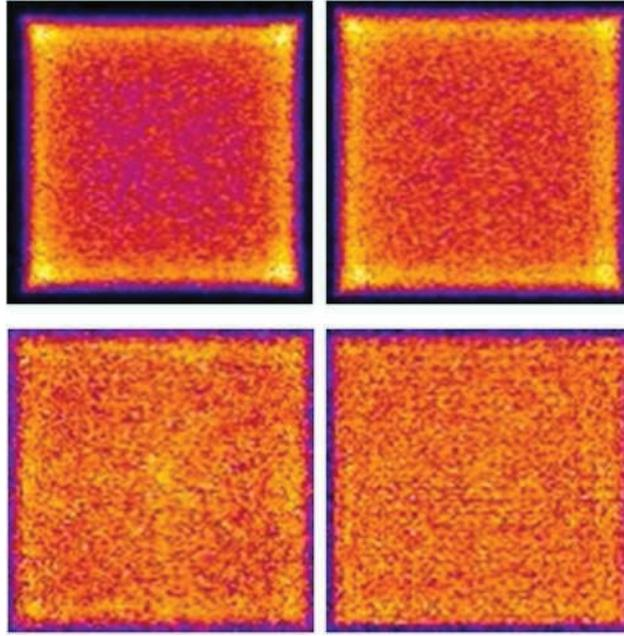
**Figure 1.** Examples of flood images reconstructed with the four algorithms. Top row: barycenter (left), barycenter squared (right). Bottom row: skewness (left), Newton (right).
