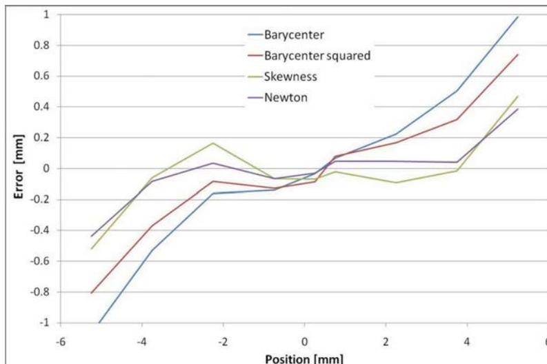
**Figure 2.** Reconstruction error as a function of the point source position for the different methods.
