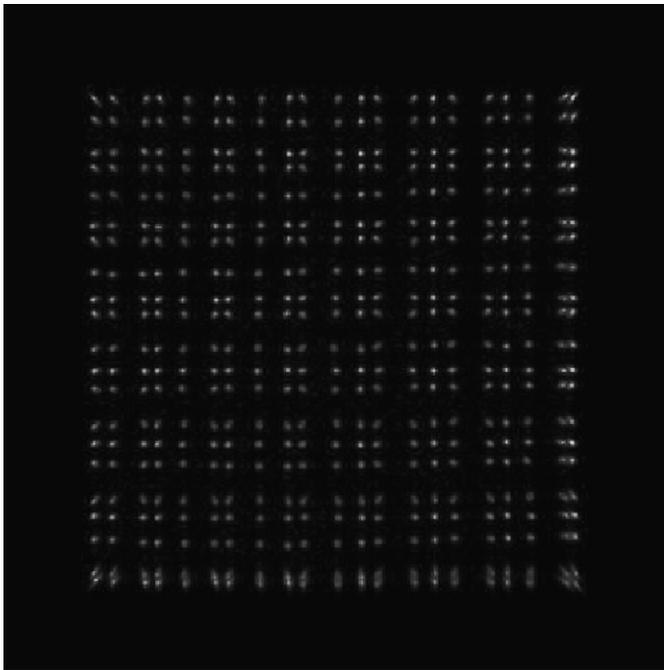
Fig. 2. Flood field  $^{22}\text{Na}$  irradiation image.  $21 \times 21$  pixels are well visible.
