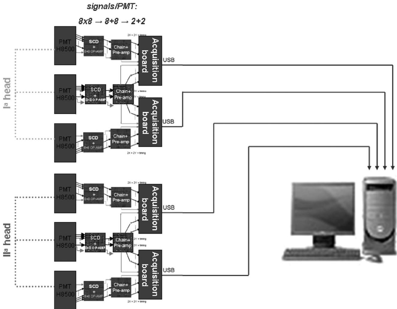
Fig. 3. Readout architecture for the entire tomograph.
