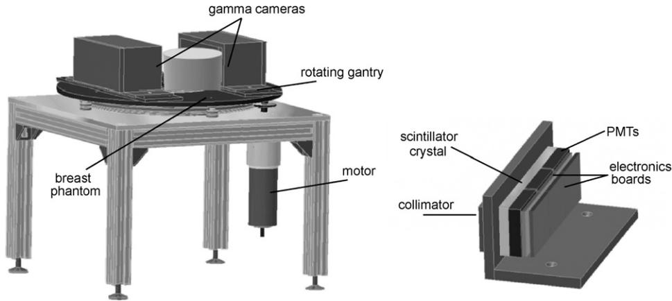
Fig. 1. Left: the mechanical assembly of the rotating SPECT ring. Right: conceptual design of a single head.
