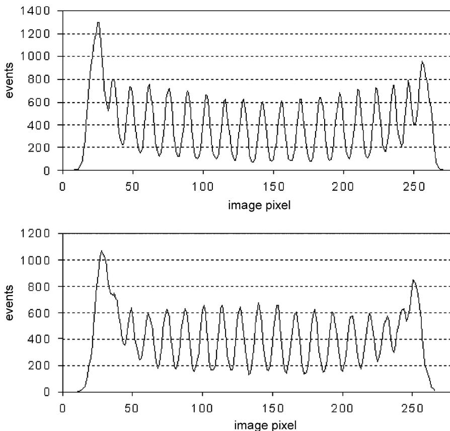
Fig. 4. Vertical profiles for a  $^{57}\text{Co}$  flood field image of one head (without collimator). Top: profile extracted from an active area. Bottom: profile extracted from a dead area.
