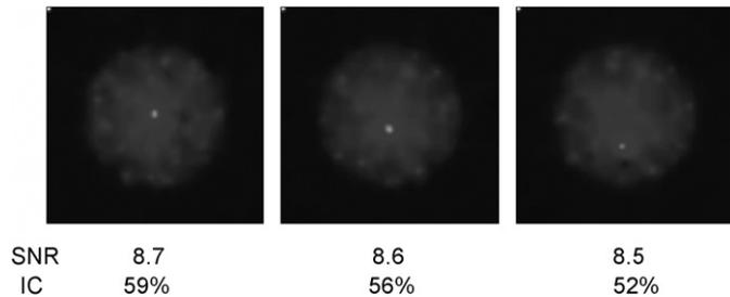
Fig. 2. Example of a reconstructed slice for an 8 mm diameter spherical tumor ( $T/B$  5 : 1) within a 10 cm diameter cylindrical breast phantom. Left: tumor on the rotation axis. Center: tumor shifted 1 cm from the rotation axis. Right: tumor shifted 2 cm from the rotation axis.
